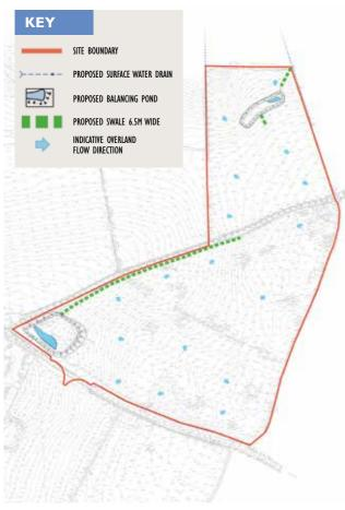
The drainage strategy we've developed focuses on providing effective drainage and management of surface water to ensure the site won't flood, while also reducing the amount of water leaving the site as run-off into surrounding area. Methods we're proposing include:
